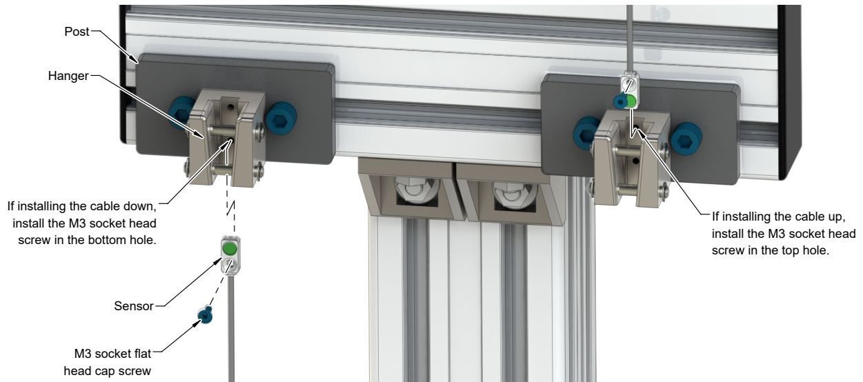
Figure 3.18—Installing Proximity Sensor for QC-7 Hook and Hanger Module
