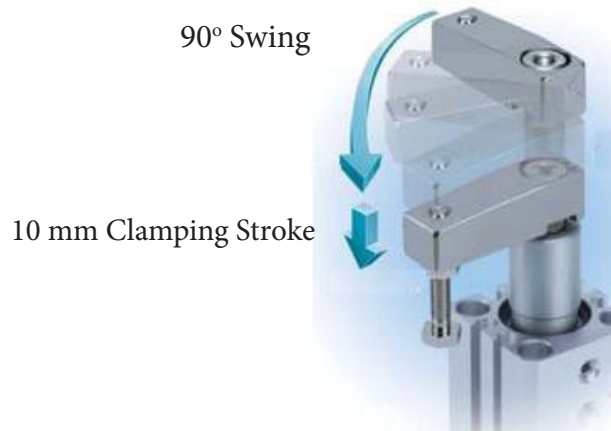
Figure 2.2—Adjustable Actuator Arm Swing and Stroke
